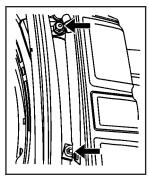
Remove the two inboard nuts from the inside of the taillamp assembly.
